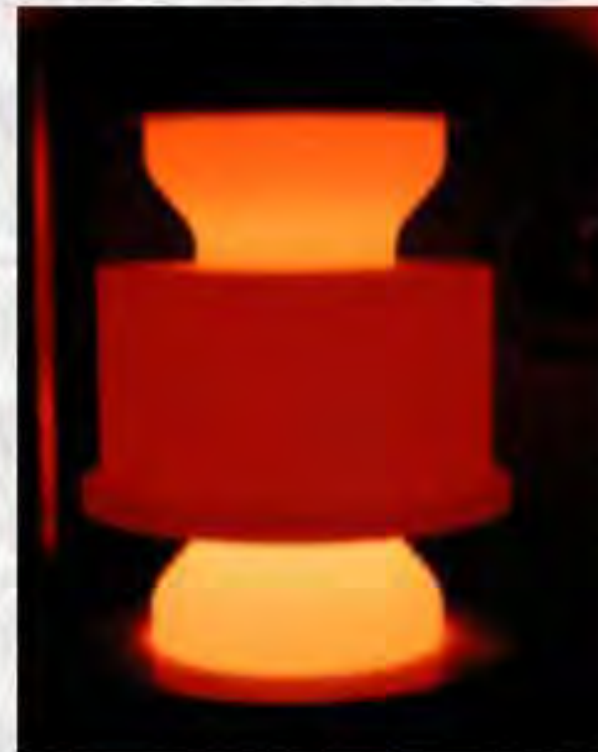
Fig. 1. Overview of the graphite set-up containing a powder sample (black), horizontal graphite papers (blue) and a vertical graphite paper sleeve (red) and a set-up during heating.
