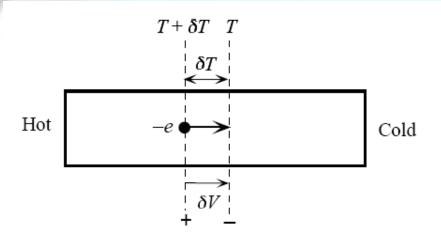
Consider a small length  $\delta x$  over which the temperature difference is  $\delta T$  and voltage difference is  $\delta V$ . Suppose that one electron diffuses from hot to cold region across this potential difference.
